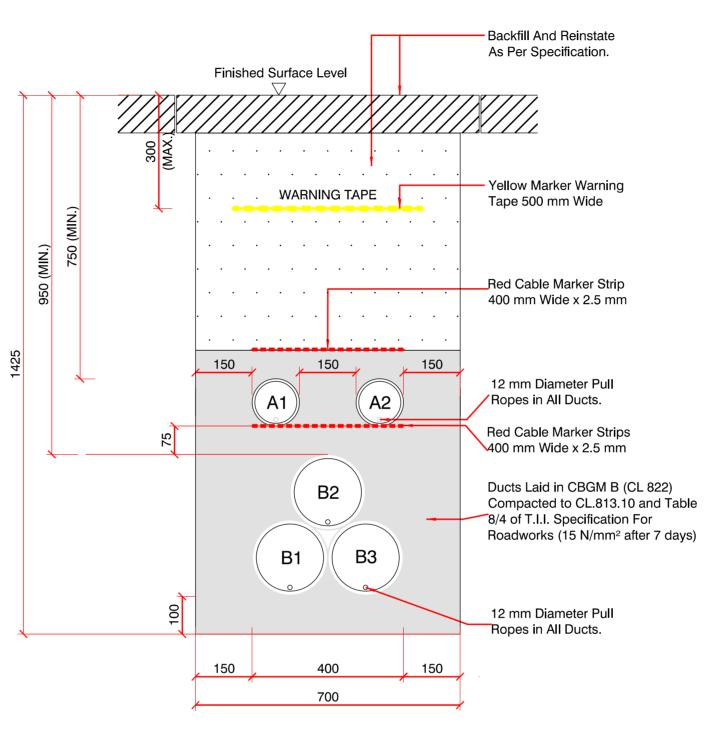
A=125 mm: Outer Diameter HDPE EirGrid Approved Duct, SDR=17.6 B=200 mm: Outer Diameter HDPE EirGrid Approved Duct, SDR=21 All Dimensions in Millimetres.
